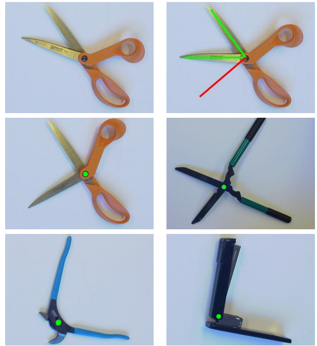
Fig. 6. Experimental results showing the manipulation of articulated objects based on interactive perception. The first row shows the scissors before the interaction (left) and after the interaction (right). The top right image also illustrates the generated manipulation plan for forming a 90^\circ angle between the blades. The second and third row show the detected revolute joints (marked with a green dot), and the results of executing the respective manipulation plans for forming a 90^\circ angle between the objects' links.
