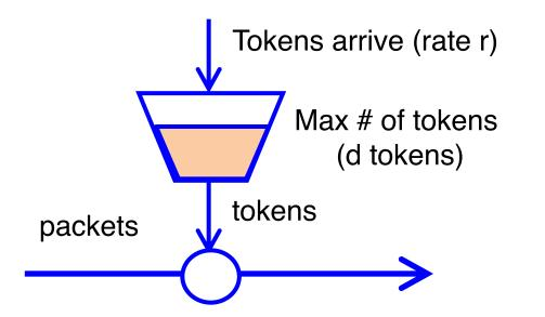
A leaky-bucket shaper for each flow or traffic class
