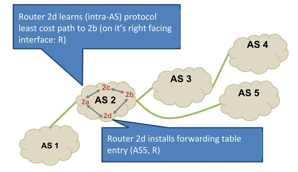
Border routers: exchange AS reachability, Internal routers: exchange intra-AS reachability., Is this sufficient to route from source to destination?
