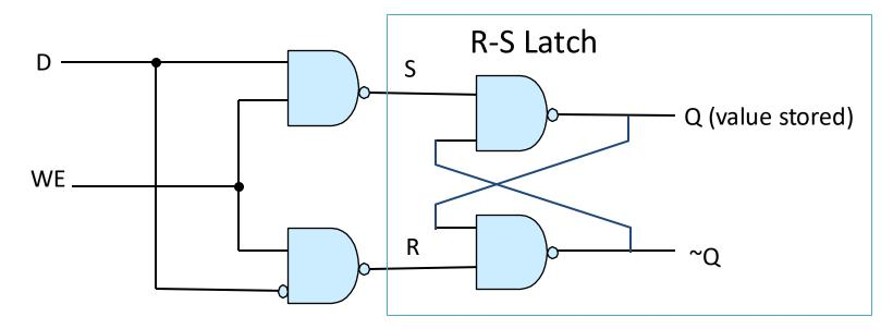
D: into top NAND, ~D into bottom NAND WE: write-enabled, when set, latch is set to value of D
