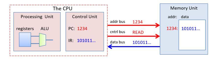
1. Fetch instruction from Memory (its addr in PC) into IR (and increment address in PC to next instruction address)
