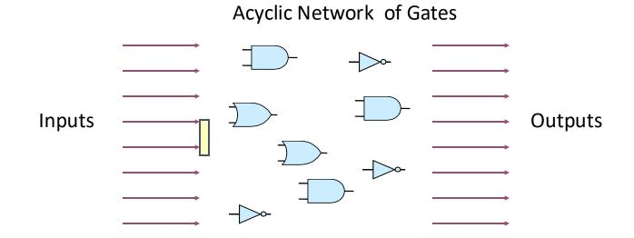
Outputs are boolean functions of inputs Outputs continuously respond to changes to inputs
