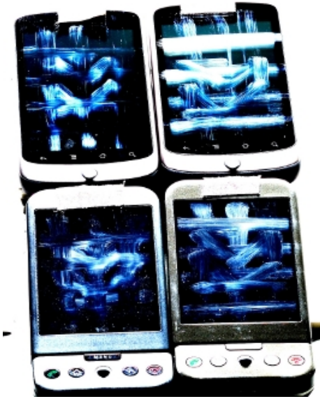
Figure A3: An image from Experiment 2: Even with background noise (over, on the left, and under, on the right of the pattern entry), either partial or complete pattern identification is possible as it contrast with such usage noise. The contrast on these images has been adjusted.
