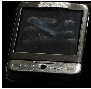
Figure 5: Phone A, from Experiment 1, where the pattern is entered with normal touches. Notice that the directionality of the pattern can be determined at ever direction change.
