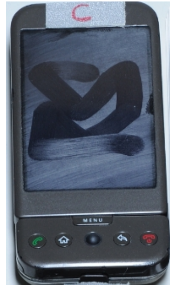
Figure A5: Phone C from Experiment 1: Without any image adjustment, the pattern is clear. Notice that the smudging, in effect, cleans the screen when compared to the broad smudging caused by facial contact. This contrast aids in pattern identification, as demonstrated in Experiment 2.
