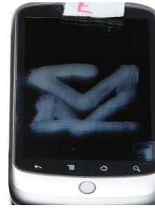
Figure 6: Phone from Experiment 3, where the phone was wiped, placed (and replaced) in a pocket. Unlike Phone A from Fig. 5, some directionality is lost in the upper left portion of the pattern.
